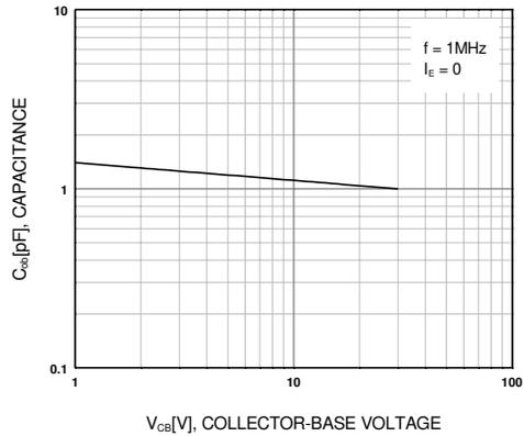
Figure 4. Output Capacitance
