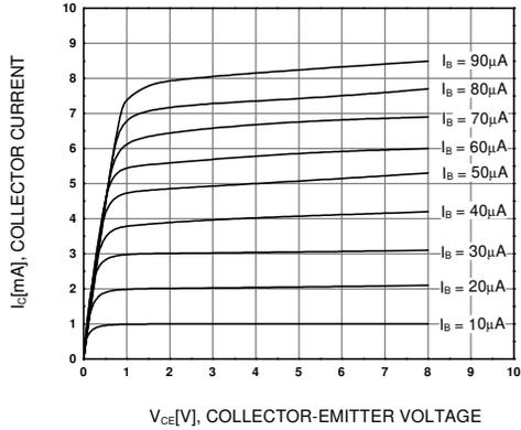
Figure 1. Static Characteristic
