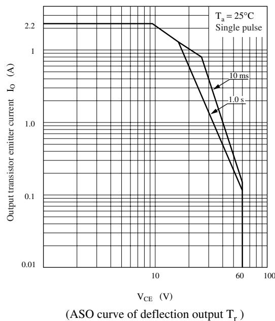
Note) The maximum value of deflection current for the actual use is suitable within  $\pm 1.5$  A[0-p] (3 A[p-p]).
