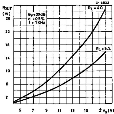
Figure 2 : Output Power versus Supply Voltage
