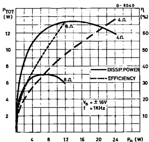
Figure 10 : Amplifier with Split Power Supply
