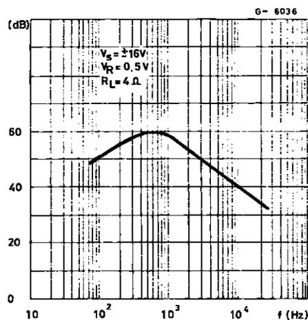
Figure 6 : Supply Voltage Rejection versus Voltage Gain
