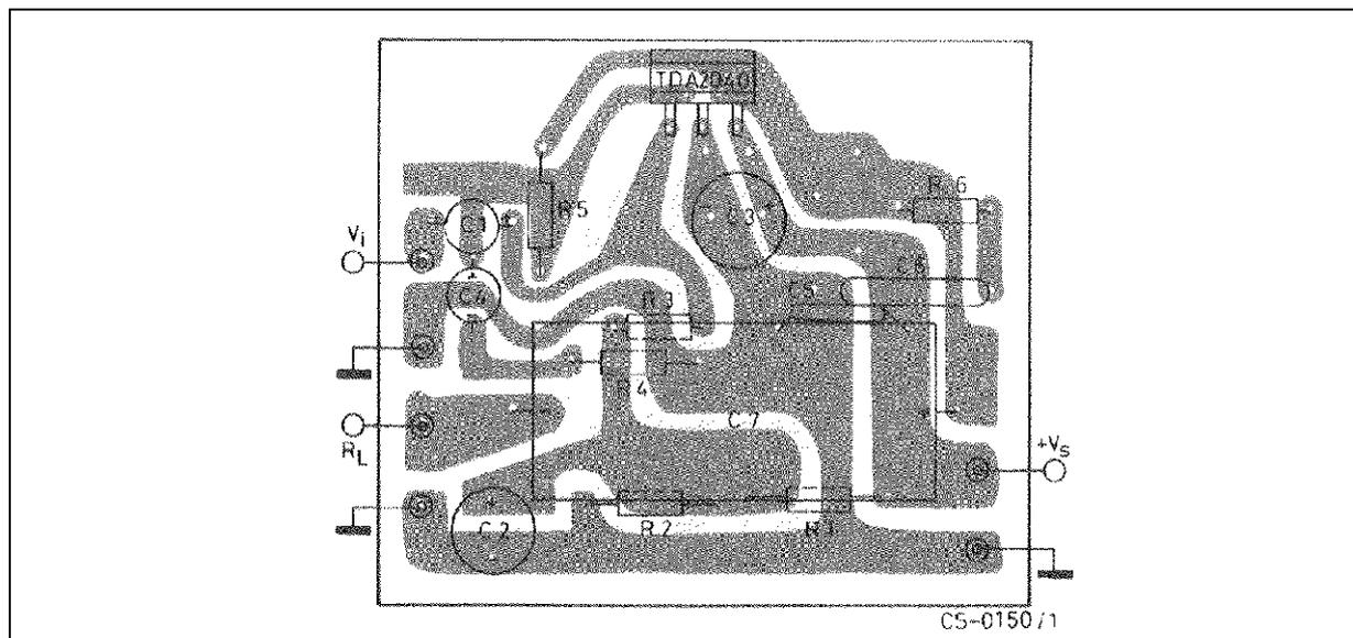
Figure 14 : 30W Bridge Amplifier with Split Power Supply
