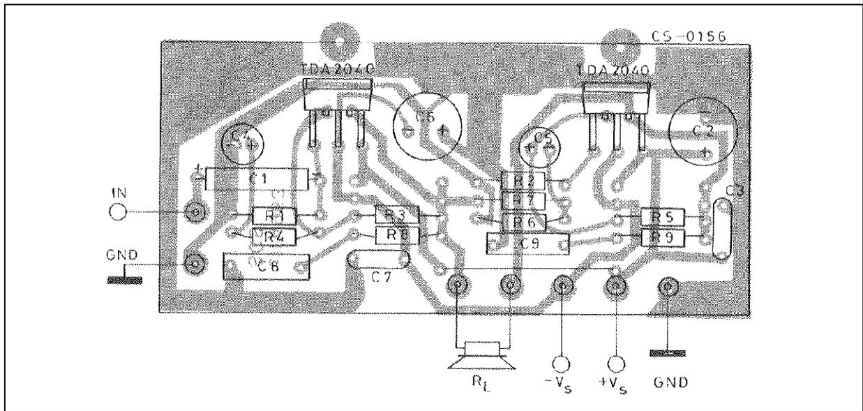
Figure 16 : Two Way Hi-Fi System with Active Crossover
