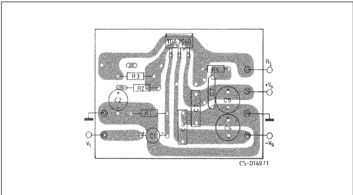
Figure 12 : Amplifier with Split Power Supply (see Note)
