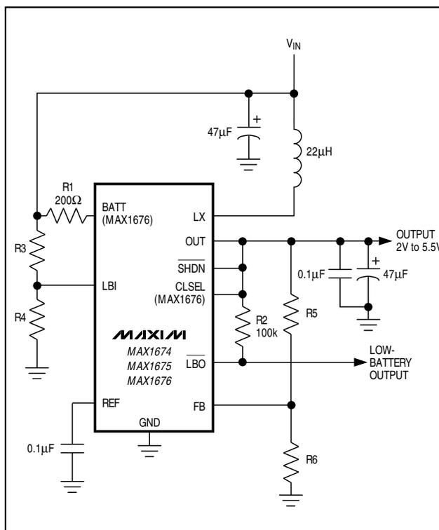
Figure 7. Setting an Adjustable Output
