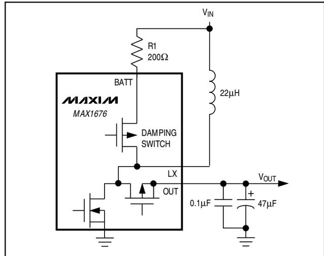
Figure 2. Simplified Diagram of Inductor Damping Switch
