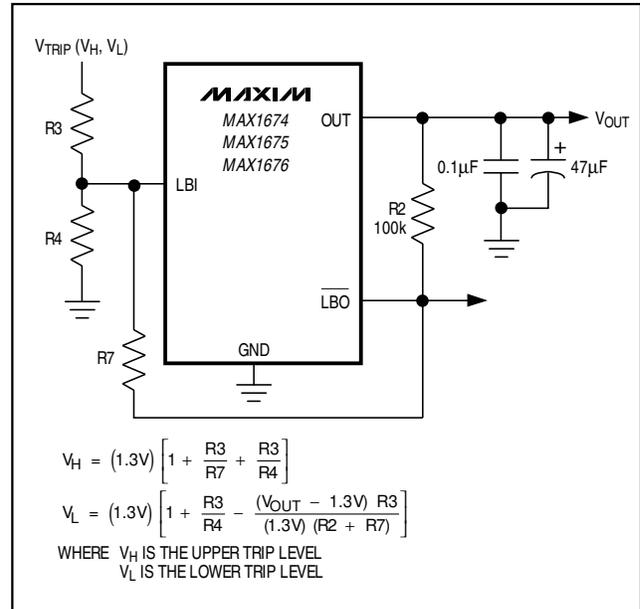
Figure 9. Adding External Hysteresis to the Low-Battery Indicator
