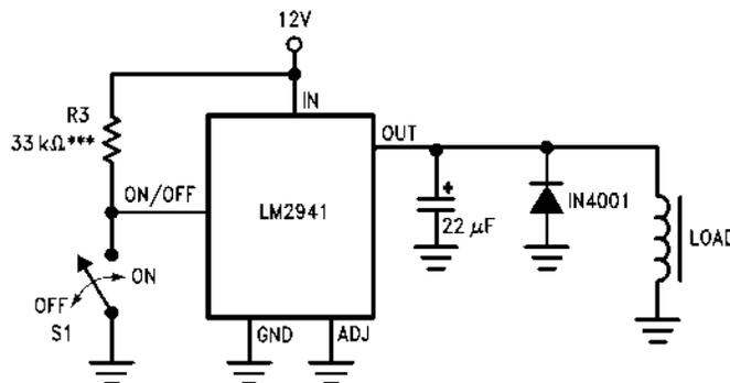
\*\*\* To assure shutdown, select Resistor R3 to ensure at least 300μA of pull-up current when S1 is open. (Assume 2V at the ON/OFF pin.)
