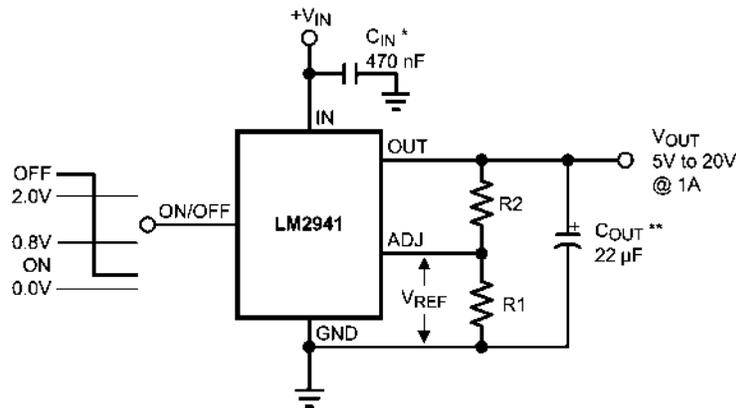
$$V_{OUT} = \text{Reference voltage} \cdot \frac{R1 + R2}{R1} \text{ where } V_{REF} = 1.2/5 \text{ typical}$$
