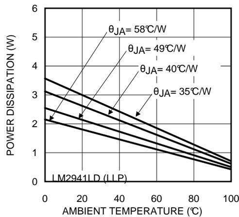
**Figure 22.  $P_{D(MAX)}$  vs  $T_A$  for LM2941LD (WSON)**
