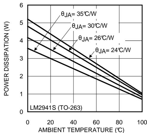
Figure 21.  $P_{D(\text{MAX})}$  vs  $T_A$  for LM2941S (TO-263)
