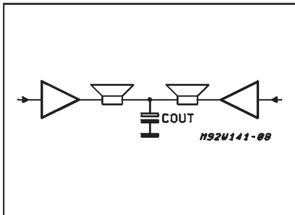
Supposing that the output capacitor  $C_{out}$  for any reason is shorted, the loudspeaker will not be damaged being this soft short circuit condition revealed.
