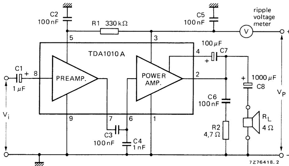
Fig.3 Test circuit.
