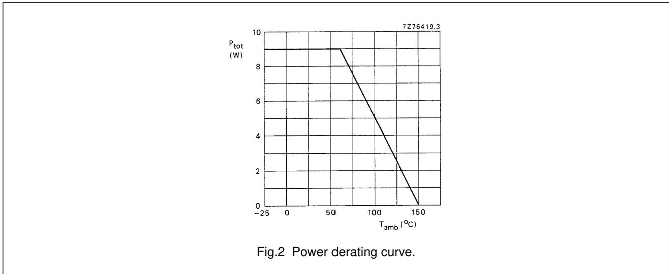
Fig.2 Power derating curve.
