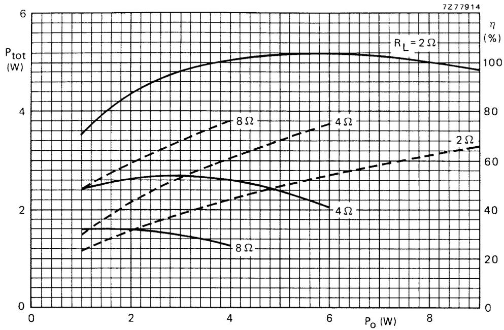
Fig.7 Total power dissipation (solid lines) and the efficiency (dashed lines) of the circuit of Fig.3 as a function of the output power with the load impedance as a parameter (for  $R_L = 2\ \Omega$  an external bootstrap resistor of  $220\ \Omega$  has been used); typical values.  $V_P = 14,4\ V$ ;  $f = 1\ kHz$ .
