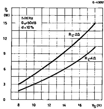
Figure 7 : Output Power vs. Supply Voltage.
