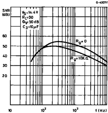
Figure 12 : Supply Voltage Rejection vs. Values of Capacitors C<sub>2</sub> and C<sub>3</sub>.
