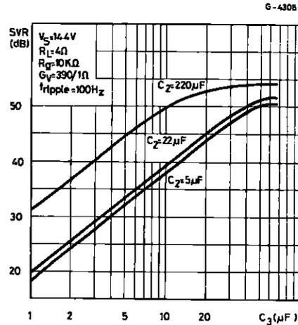
Figure 13 : Supply Voltage Rejection vs. Values of Capacitors C<sub>2</sub> and C<sub>3</sub>.
