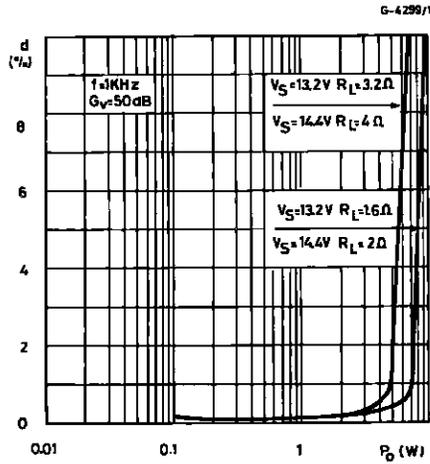
Figure 6 : Output Power vs. Supply Voltage.
