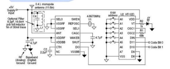
Figure 2a. 315MHz, 1kbps On-Off Keyed Receiver/Decoder
