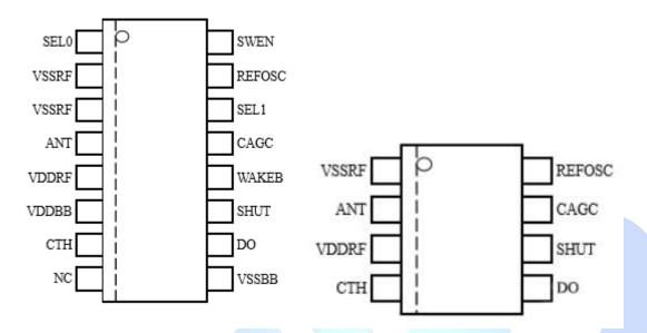
Standard 16-Pin or 8-Pin SOP (M) Packages
