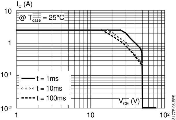
**Figure 2 :** Secondary Breakdown Temperature Derating Curve
