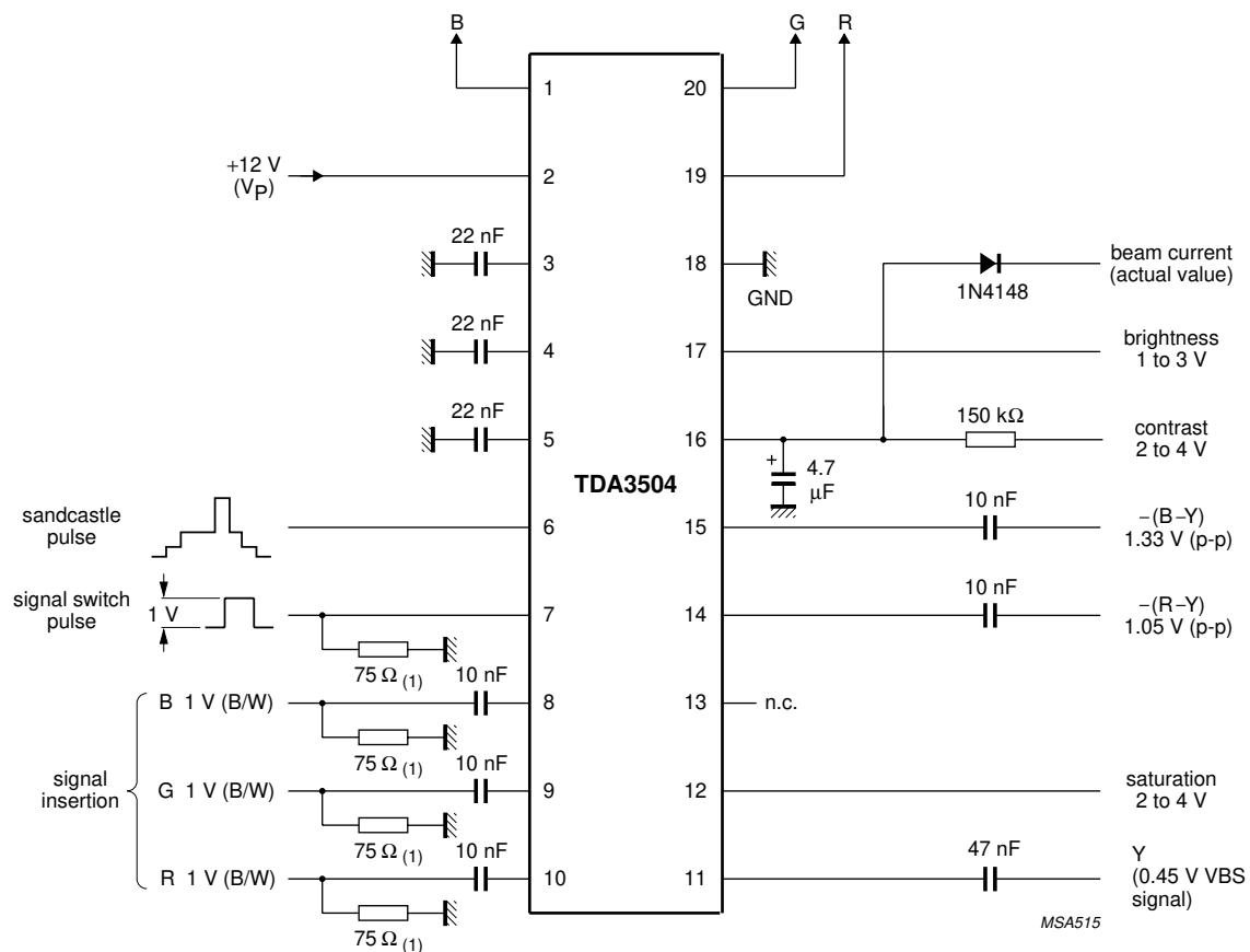
Fig.3 Basic application circuit diagram.
