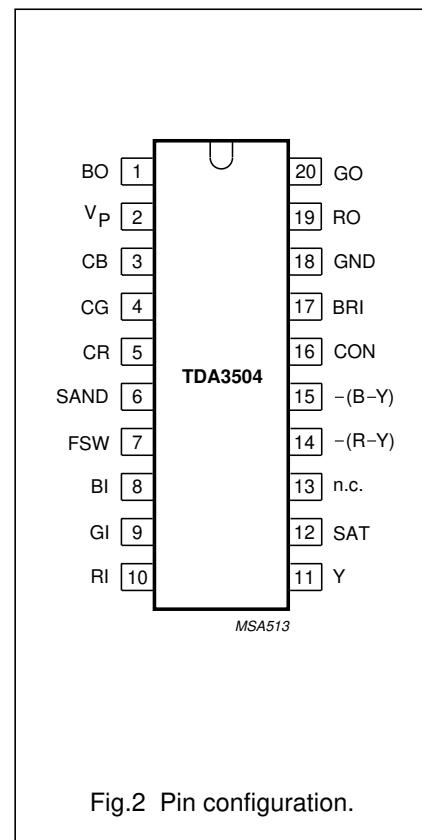
Fig.2 Pin configuration.
