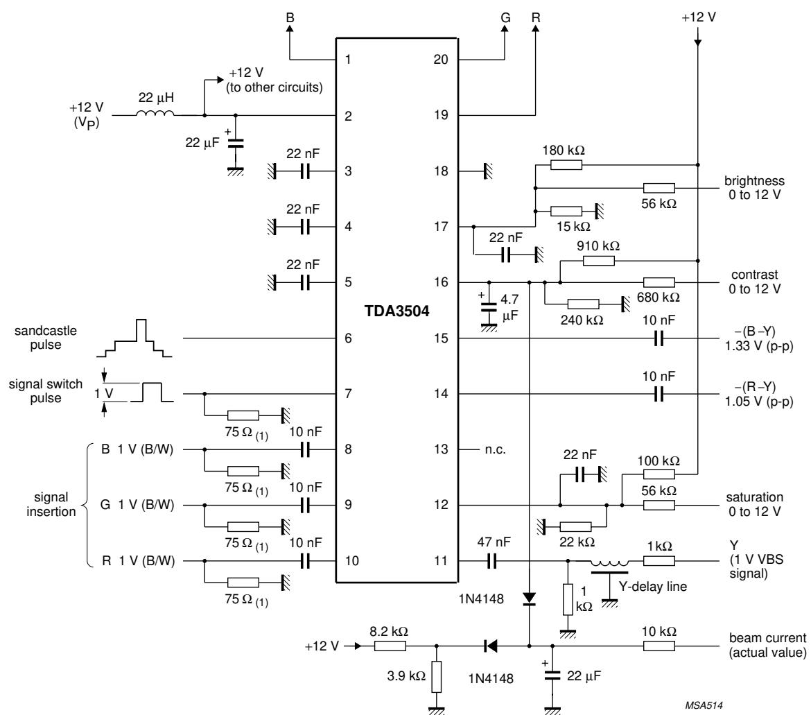
Fig.4 Typical application circuit diagram.
