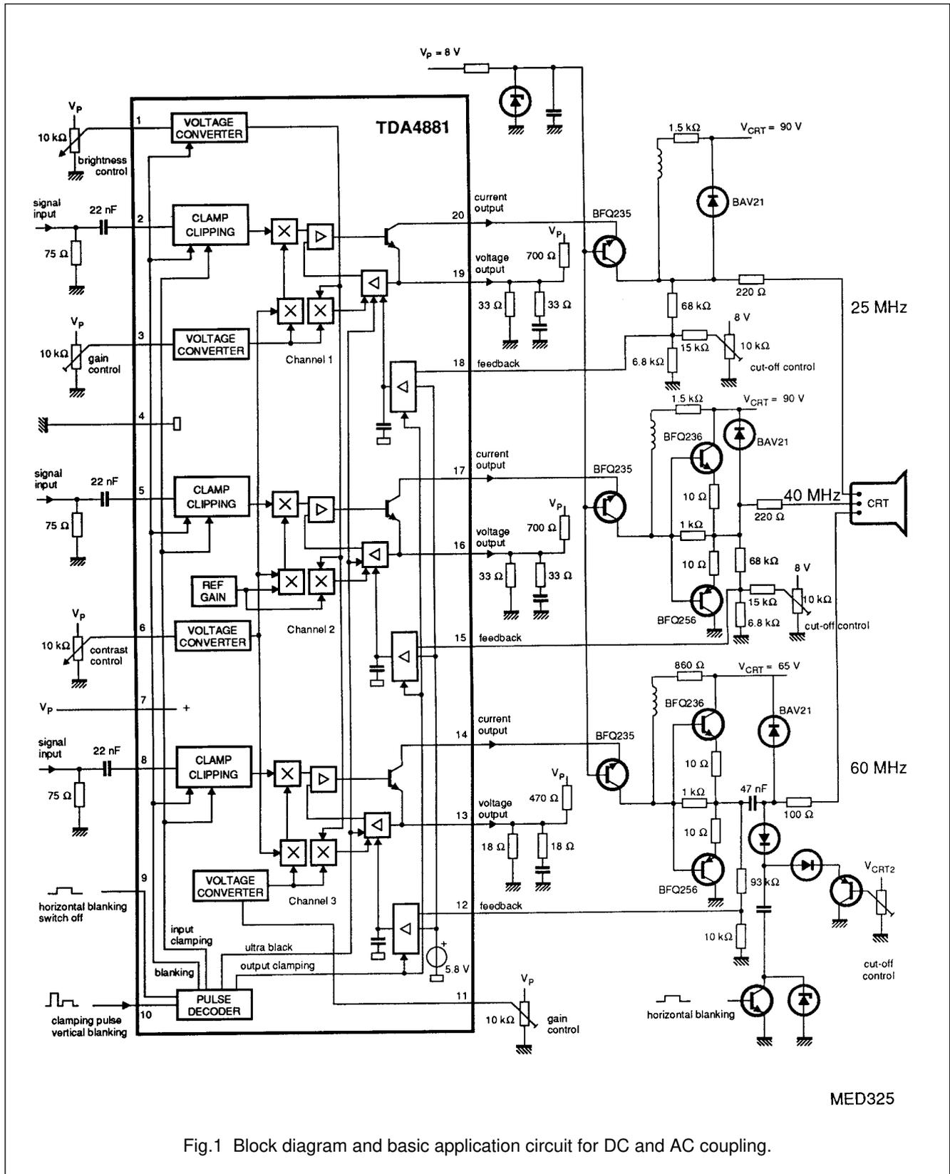
Fig.1 Block diagram and basic application circuit for DC and AC coupling.
