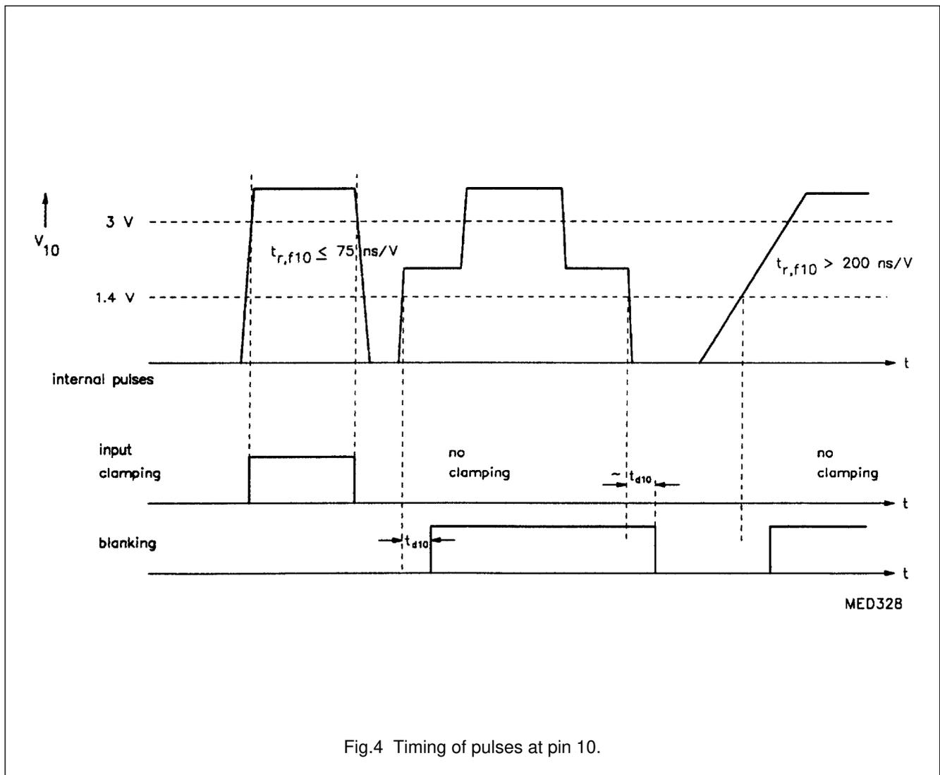
Fig.4 Timing of pulses at pin 10.
