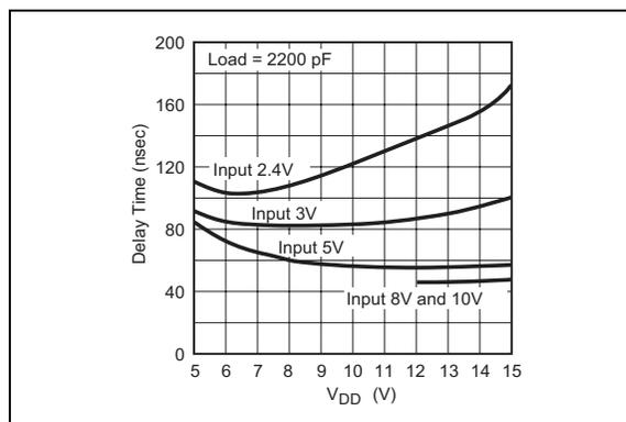
**FIGURE 2-11:** Effect of Input Amplitude on Propagation Delay.
