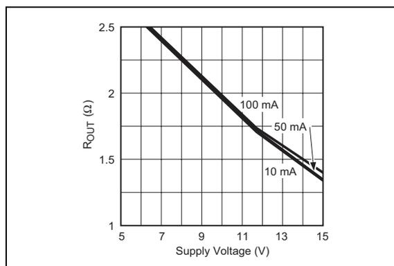
**FIGURE 2-12:** Low-State Output Resistance vs. Supply Voltage.
