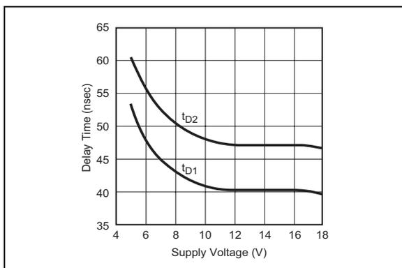
**FIGURE 2-8:** Propagation Delay Time vs. Supply Voltage.
