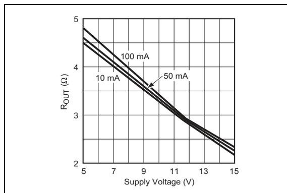
**FIGURE 2-10:** High-State Output Resistance vs. Supply Voltage.
