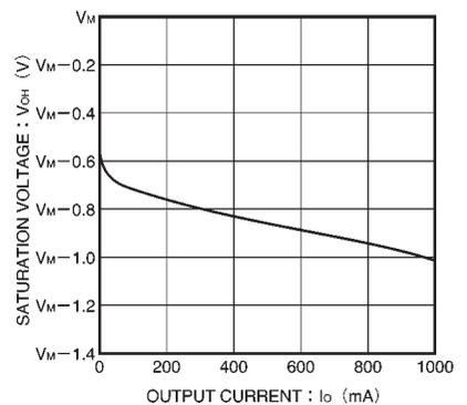
Fig.16 Upper-side output saturation voltage vs. output current
