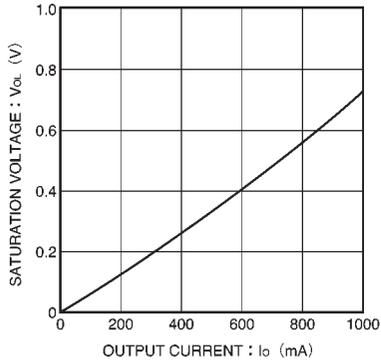
Fig.17 Lower-side output saturation voltage vs. output current
