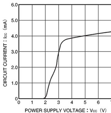
Fig.15 Power supply current vs. power supply voltage
